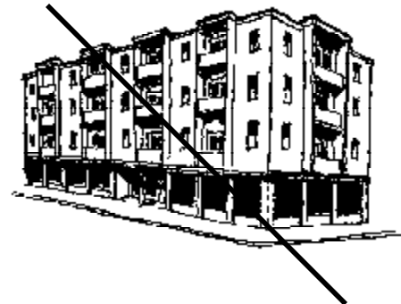
FIGURE 11. The void to solid ratio is disrupted by facades that are primarily glazed and by a predominance of balconies.
